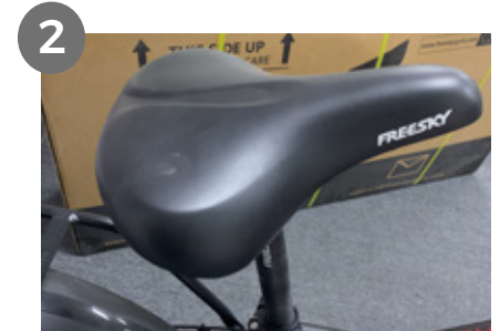
2. Move the seat up and down by sliding the seatpost in or out of the seat tube. DO NOT raise the seatpost beyond the minimum insertion marking etched into the seatpost tube.
