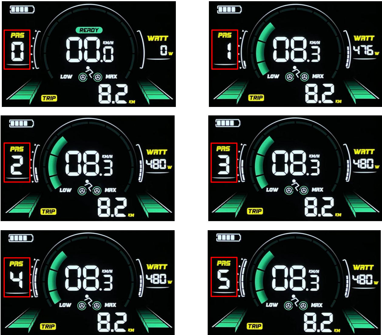
Figure 5-5: Level Switch Display
