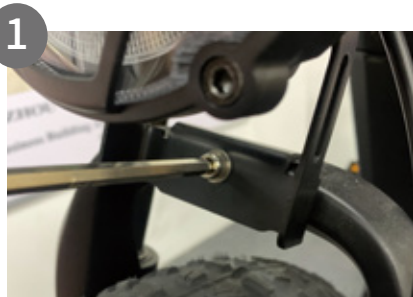
1. Put the headlight on the arch of the fork. Locate the bolt hole.
